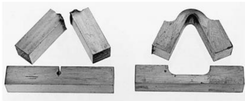
FIGURE 1-14 Notched and unnotched impact specimens before and after testing. Both specimens had the same cross-sectional area, but the notched specimen fractures while the other doesn't
